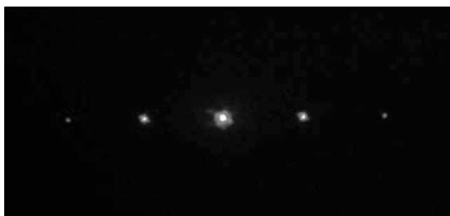
FIGURE 6 A diffractive pattern of a readout beam after it propagates across the holographic gratings illustrated in Figure 5. The readout beam, operating at 633 nm, is provided by a HeNe laser.
